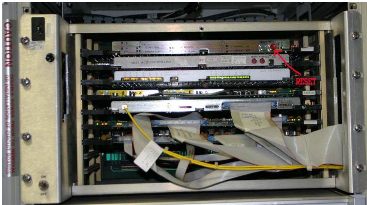
UNITY600 Plus Console RESET button position.
